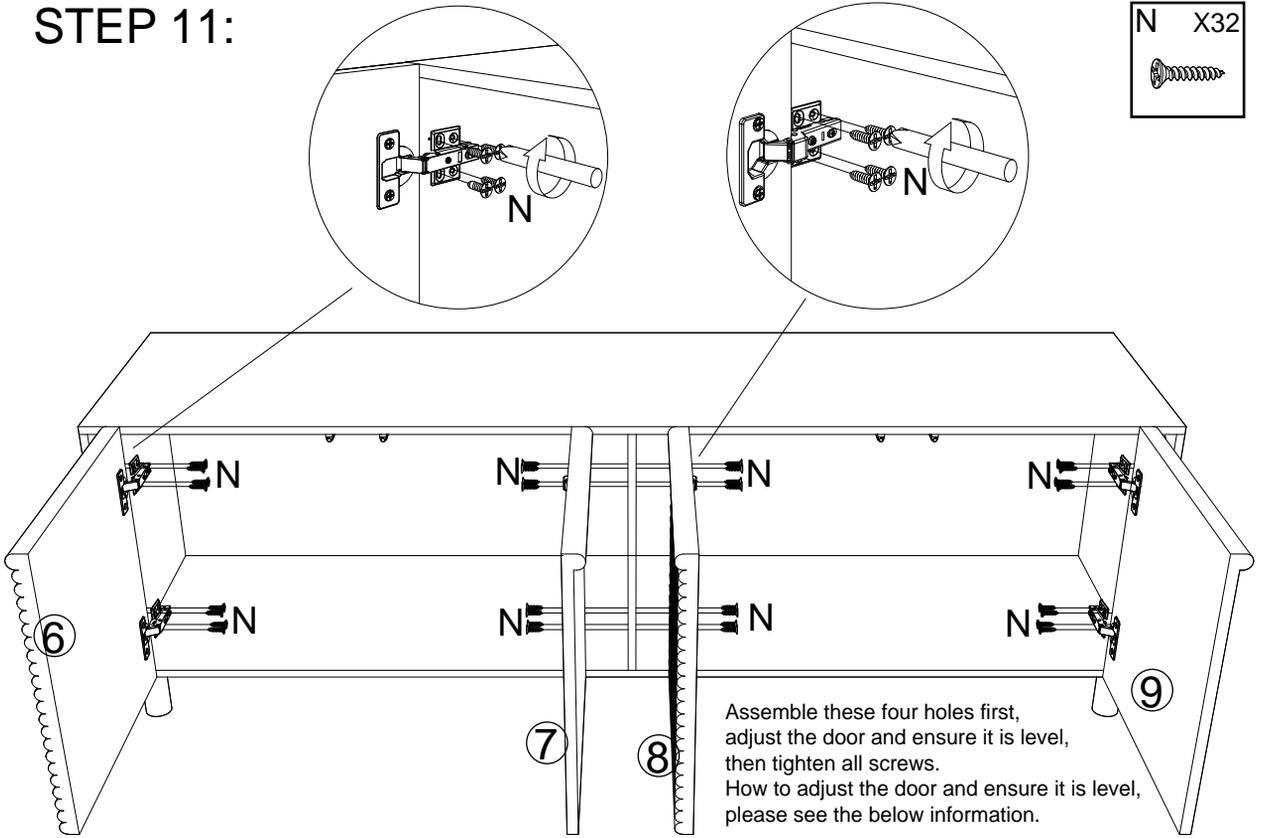
Assemble these four holes first, adjust the door and ensure it is level, then tighten all screws.
